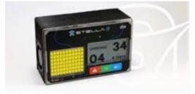
Your request has sent an alert to the vehicle ahead and his LEDS monitor will start flashing blue, followed by an alert sound or beep. This condition will continue until the competitor ahead authorizes the pass.
