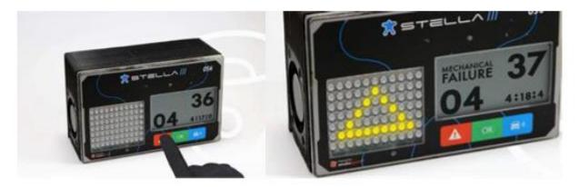
Competitors approaching your vehicle with mechanical failure will receive an alert on their led monitor, a symbol in the shape of flashing red triangle and an alert sound or a beep when they are within 300m of the damaged vehicle.
