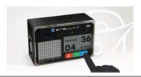
Your LEDS monitor will flash in yellow color to indicate that the vehicle you are attempting to pass has not received your request for passing. When the yellow monitor stops flashing, it indicates that the vehicle ahead has already received your request for passing.
